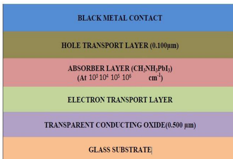
Figure 3: Perovskite Solar Device Model with Different Absorption Coefficient of (cm -1 )
